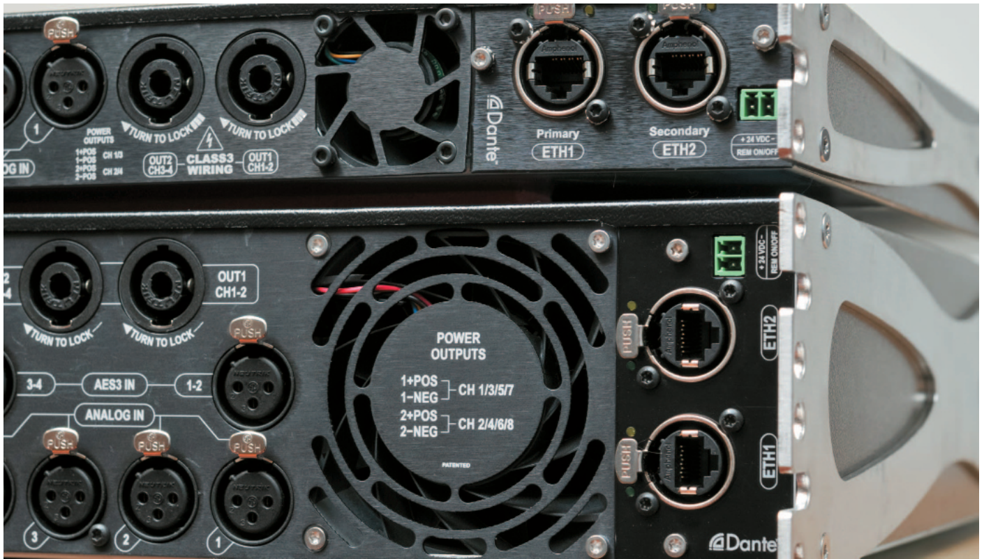
Network sockets for the primary and secondary connection of a Dante network. Above the X4, below the X8
